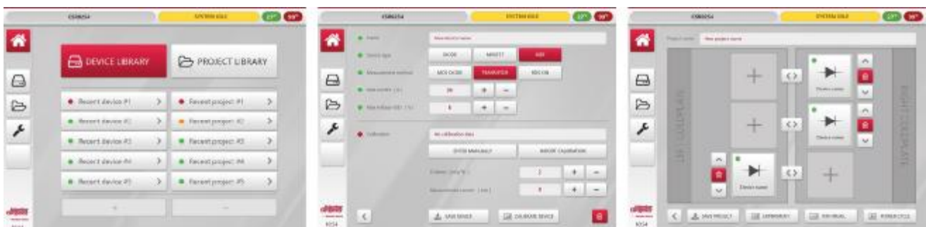
Figure 3: The Power Tester 1500A touch-screen interface (left to right): main screen, device creation, and placing devices on the cold plate.
