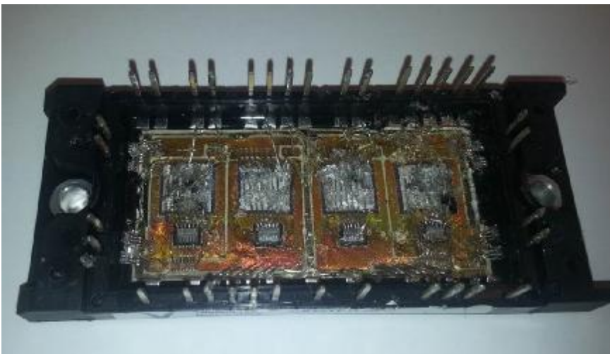
Figure 1: Damaged IGBT modules.
